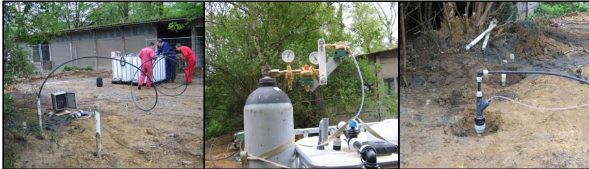
Figure 3. Picturing during the pilot test. Left: groundwater is extracted and captured in a container (pull). Middle: Purging with nitrogen during mixing. Right: re-infiltration of mixture under constant nitrogen purging (push)
